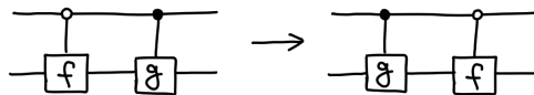
Figure 11: One of the equations on control in quantum circuits, presented as a rewrite rule.
